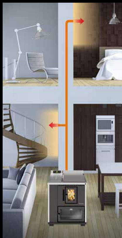
Canalization air chaud
